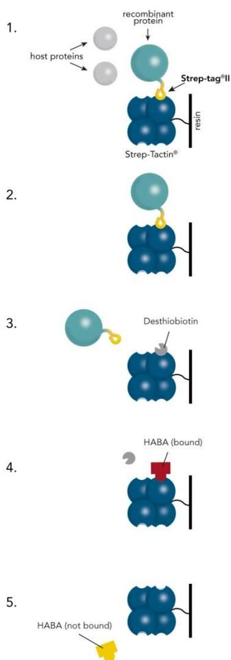
**Steps 1 + 2:** The sample is added to the column. Once the tagged protein has bound specifically to Strep-Tactin® the host proteins are washed away rapidly with small amounts of physiological wash buffer (Buffer W).
