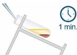
**3.2.2.** Incubate the tube on a magnet for **1 min**, remove entire supernatant carefully.
