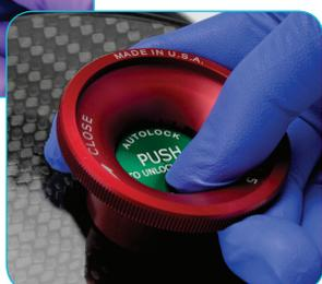
Auto-Lock is identified on Thermo Scientific superspeed centrifuges with a **black push button** and on Thermo Scientific general purpose and small benchtop centrifuges with a **green push button**.
