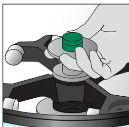
Push center button to remove rotor
